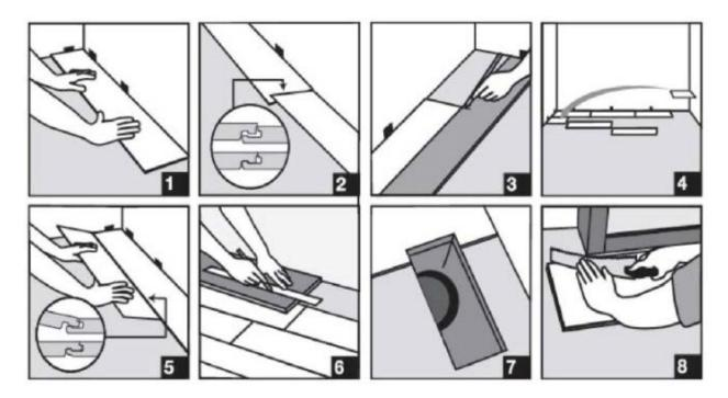
Diagram 1. Start in a corner by placing the first plank with the tongue side facing the wall. Use spacers along each wall to maintain an expansion space of 3/8" - 1/2" (8-12mm) between the wall and the flooring. NOTE: This spacing must also be maintained between the floor and all vertical surfaces, including, cabinets, posts, partitions, door jambs and door tracks. You will also need to use transition strips in doorways and between rooms. Failure to do so may cause buckling or gapping.
