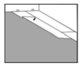
NOTE: The lock joints cannot be 'lifted' or angled apart when removing or repositioning a plank. To remove a plank, first disengage the top/long angle joint by lifting at a slight angle while pulling the complete rows away from each
